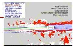
Course overview generated from Stanley's laser sensor data as the robot navigated Beer Bottle Pass
