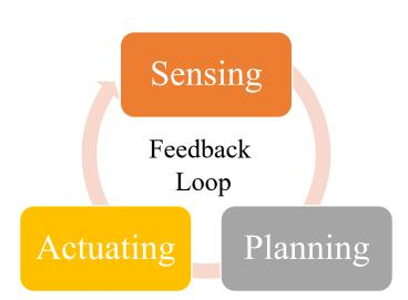
The sensors feed measurements to a controller or computer, which processes them and then sends control signals to motors and actuators.
