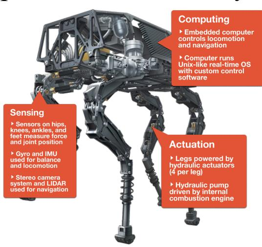
BigDog, a rough-terrain quadruped robot developed by U.S. firm Boston Dynamics.
