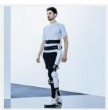
**Exoskeletons:** Robotic exoskeletons can be used for physical rehabilitation and for enabling a paralyzed patient walk again. Some have industrial or military applications, by giving the wearer added mobility, endurance, or capacity to carry heavy loads.
